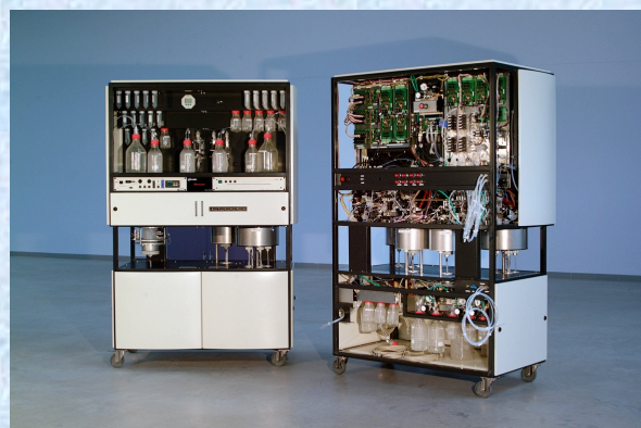
An industrial realization of the Synthesizer of Small Organic Molecules in combinatorial chemistry, solid phase
